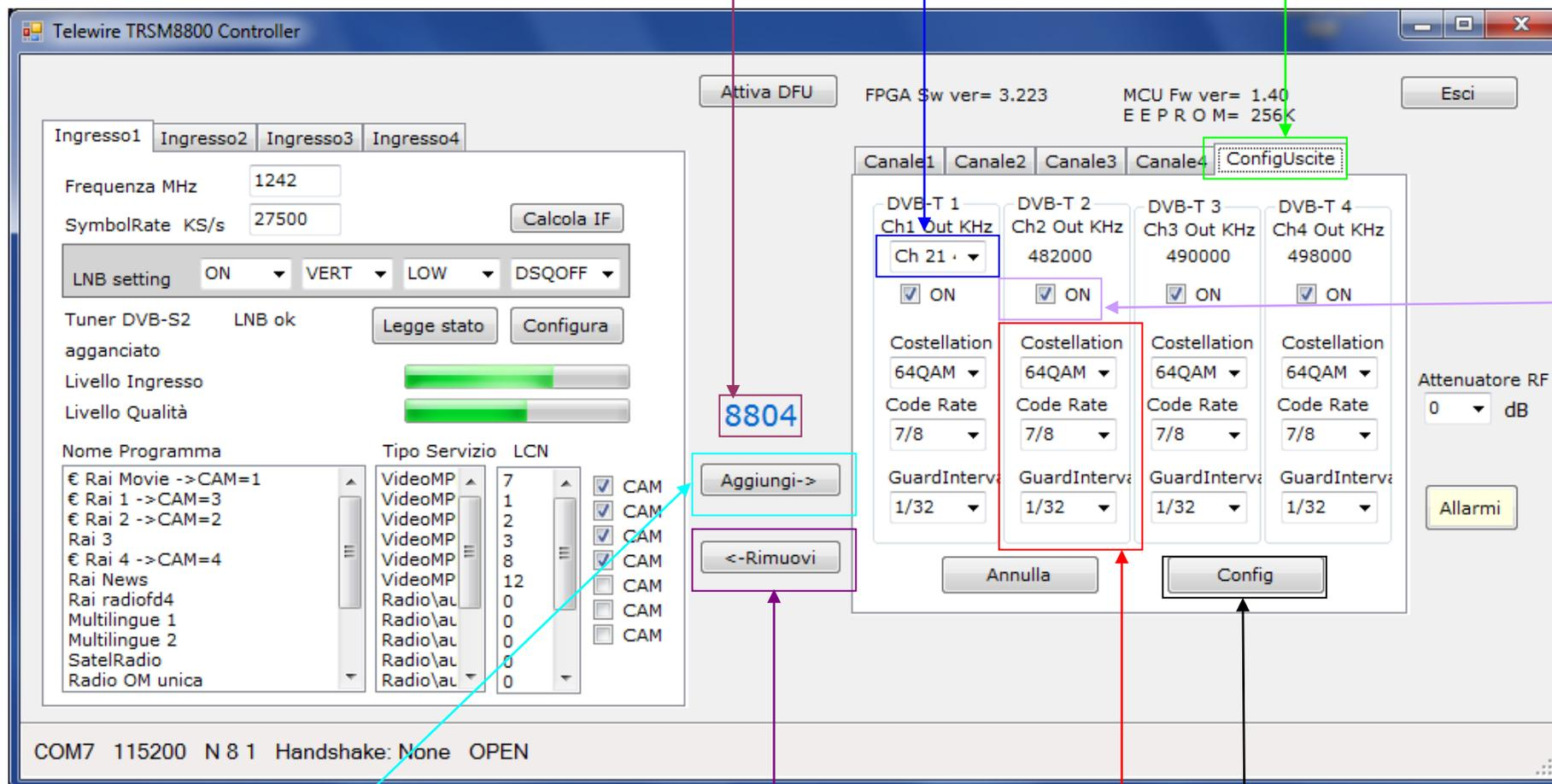
The screenshot shows the 'Telewire TRSM8800 Controller' window. At the top, it displays 'Attiva DFU', 'FPGA Sw ver= 3.223', 'MCU Fw ver= 1.40', and 'E E P R O M= 256K'. Below this are tabs for 'Ingresso1' through 'Ingresso4' and 'Canale1' through 'Canale4', along with a 'ConfigUscite' button. The main area is divided into several sections:
